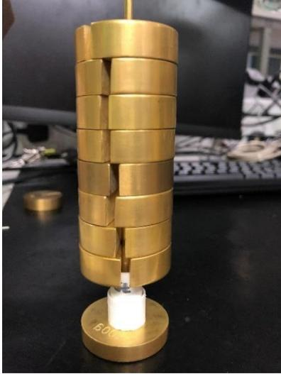
*Figure 1. Test setup for estimating the friction force due to the seal*
