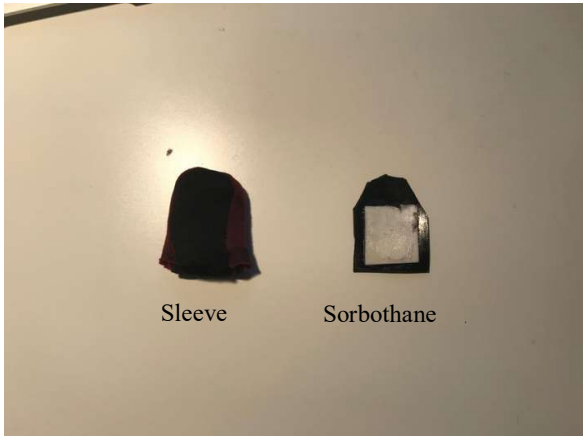
Figure 46. Vibrating motors sleeves
